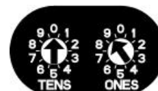
Figure 28: B208 Switches Set to Address 9
