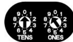
Figure 29: B308 Switches Set to Address 9
