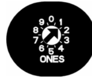
Figure 30: B420 Switch Set to Address 1
