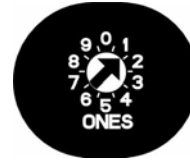
Figure 31: B820 Switch Set to Address 1
