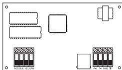
This Escort5580 module will turn any touch tone phone into a fully functional keypad. The module also includes a built-in interface to control up to 32 line carrier type devices for lighting and temperature control (See [Section 5.28 "Escort5580 Module"](#)). (See [Escort5580 Installation Manual](#).)
