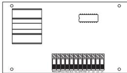
The PC5204 can provide up to 1 Amp of additional power for modules or devices connected to the control panel. The module requires a 16.5 volt AC 40 VA transformer and 4 AH battery. In addition, the module provides 4 programmable high current voltage outputs. Each output is individually programmable with 14 different output options available (See [Section 5.10 "PGM Outputs"](#)). (See [PC5204 Installation Instructions Sheet](#).)
