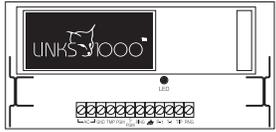
The LINKS1000 Cellular Communicator provides an efficient, cost-effective method for adding cellular back up. The unit comes in its own cabinet with antenna and requires a separate battery and transformer (See [Section 5.26 "LINKS1000 cellular communicator"](#)).
