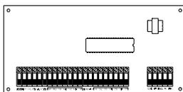
The PC5928 Audio Interface module is a simple way to incorporate paging, intercom, baby listen-in and door answer to the PC5010 control panel. The module also has built-in two-way voice capability for central station (See [Section 5.30 "Audio Interface Module"](#).)
