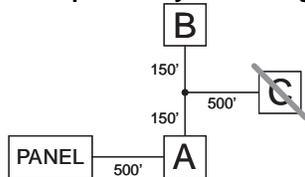
NOTE: Module (A) is wired correctly as it is within 1,000'/330m of the panel, in wire distance.
