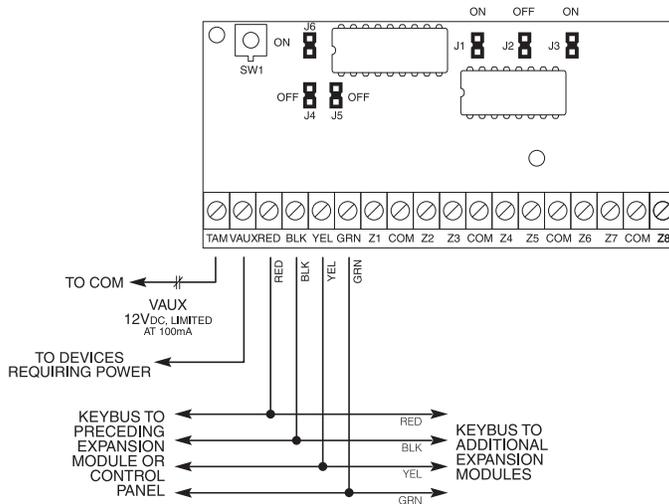
In the above diagram the jumper settings shown indicate the first group of four zones of the expander will be zones 9 to 12 and the second group of 4 zones will be 13 to 16.
