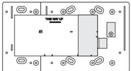
This backplate is to be used when an Audio Station is to be located next to a keypad. In addition to the backplate will allow you to mount a PC5108 Zone Expander Module or the PC5208 Eight Low Current Output Module. Dimensions 208mm x 115mm x 18mm / 8.2" x 4.5" x 0.7" approximately.
