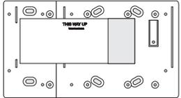
This backplate is to be used when an Audio Station is to be located next to a keypad. Dimensions 208mm x 115mm x 18mm / 8.2" x 4.5" x 0.25" approximately.
